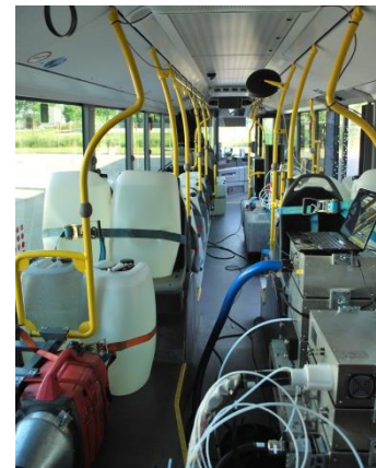
Figure 3: PEMS analyzers, additional equipment and payload inside the bus.
